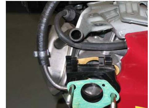
5) Install insulator equipped with pulse line and gaskets in the same orientation as they were removed
